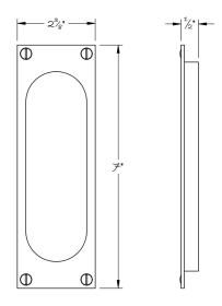
The No.3107 rectangular flush pull is available with face mounted fasteners or concealed screws.
