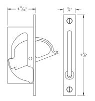
An elegant design with only one moving part and no springs. Simply push bottom of the rotating pull in and the top pops out. Gravity constantly wants to rotate pull back down to its stored position. Case measures 1/2" thick. Square or round faceplate ends available. Available in all finishes.
