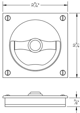
*The #3100 drop ring pull is a marriage of 3 fully CNC machined components that work in perfect unity to maintain beauty and function. The ring swells slightly at its midpoint to enable a sure grip. Selective stainless steel wave springs between the ring and decorative hub keep the piece from rattling while under way out to sea.*
