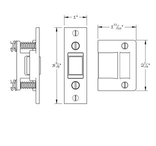
The #210 roller latch is adjustable in its force of engagement. The rubber roller engages the strike and holds the door firmly closed without any unnecessary loud clicks.
