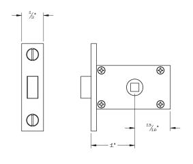
The Lowe Hardware No. 2000 mortise latch for cabinet doors with a minimum thickness of 3/4".
