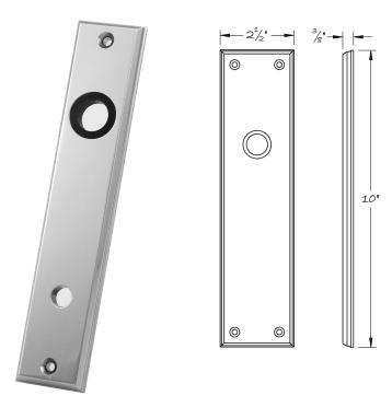
Featured in our Alphecca suite, the #1506 features a chamfered edge that is proud of a small cove around the perimeter. The plate can be machined for use with American or European locks, latches, or screen door hardware, or simply as a push plate.
