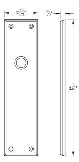
Featured in our Alphecca suite, the #1506 features a chamfered edge that is proud of a small cove around the perimeter. The plate can be machined for use with American or European locks, latches, or screen door hardware, or simply as a push plate.
