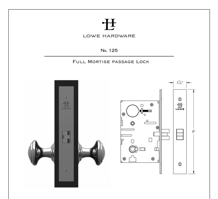
The Lowe 125 full mortise passage lock is available in 2–1/2", 2–3/4", 3–3/4", 5" or 6" backsets. The 125 is typically used on passage doors that require a listed lockset. The lock can be configured at the factory to be used with knobs, levers, thumblatches or any combination thereof. It is supplied with a strikeplate and stamped metal dustbox, and the faceplate has an adjustable bevel. The 125 is ANSI Grade 1, and is UL listed with a 3 hour fire rating. Available in all finishes.
