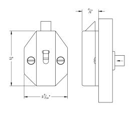
Lowe Hardware's #1092 push button drawer latch is known for its simplicity of use and robustness in a sea way. Machined from solid brass, the body features a 5/8" diameter pilot which aligns the latch with the outer trim ring. A simple push of the buttondraws the tongue down, and the spring latch function allows "slam" closing.
