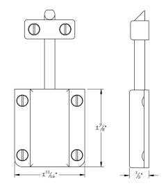
Similar to the #1080, the #1081 drop panel latch has a guide bracket designed for panels not mounted to drawer boxes. Routing out for the strikeplate is required and shown in the picture.
