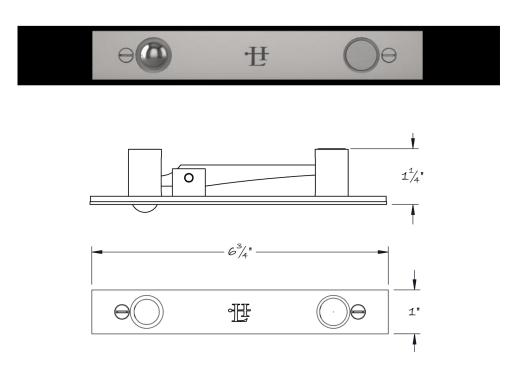
An ideal solution for larger hanging locker doors on yachts or any other smaller double door application in bathrooms, offices, and master baths.
