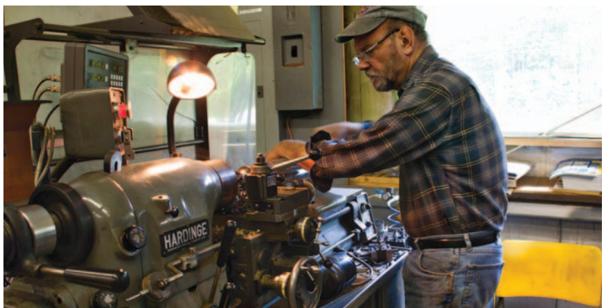
Bill Lowe shapes a piece of equipment on a manual lathe. He often designs custom tools to facilitate different designs.
