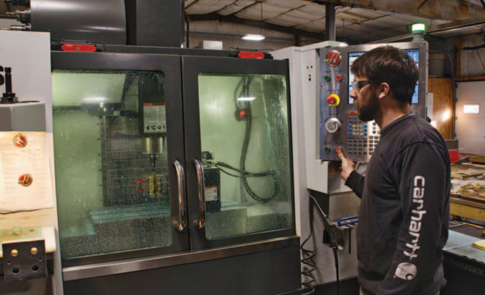
An employee watches as a computer-controlled cutting machine creates a door hinge.
