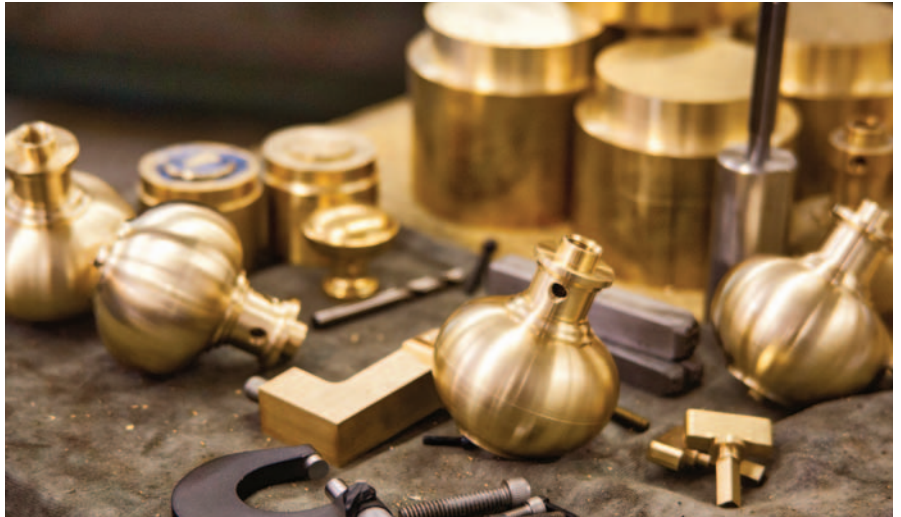
Jewel-like bronze knobs in the foreground are fashioned from solid rods, shown here in the background. The Lowes cut hardware out of solid metal, rather than casting or forging it.
